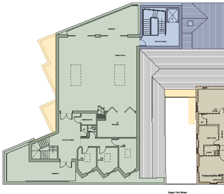
Phasing Proposed Second Floor Plan All phasing to allow two ways of escape at any given time up to phase 3
